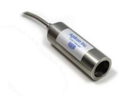
Agiltron's 1kW (CW) Fiber Collimators incorporates advanced technologies of direct fusion to a large beam expanding end cap ensuring safe power density, and a mode stripper that prevents burning the buffer/jacket by removing unwanted back-reflection radiation. These technologies significantly increase the collimator reliability.
